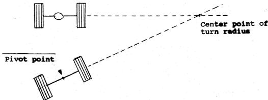
Figure 9 – Single pivot turning radius
