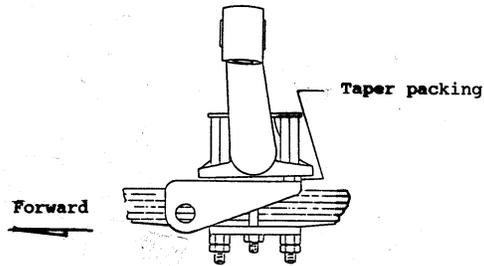
Figure 8 – Taper packing to change caster angle
