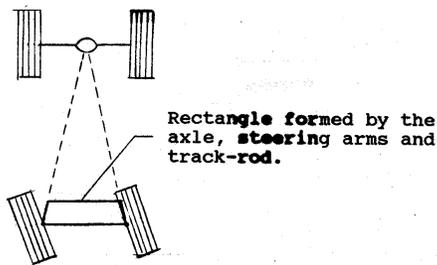
Figure 10 – Ackerman steering principle
