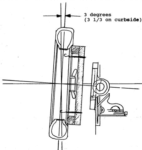
Figure 11 – Simple measuring device
