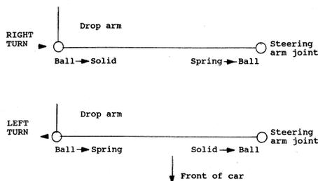
Figure 4 – Transmission of forces
