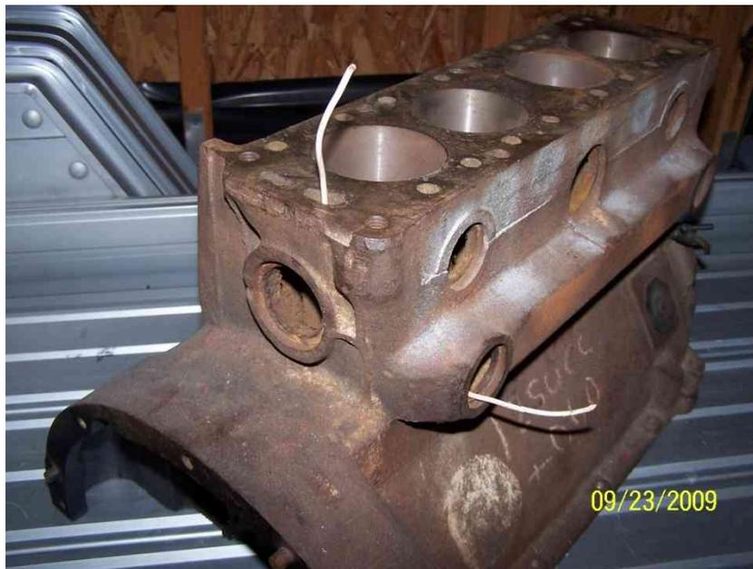
When the water exits the top of the block it goes into the head. As you can see the water comes in through the large opening at the rear of the head and into this chamber which connects to a passage that runs all the way through the head.
