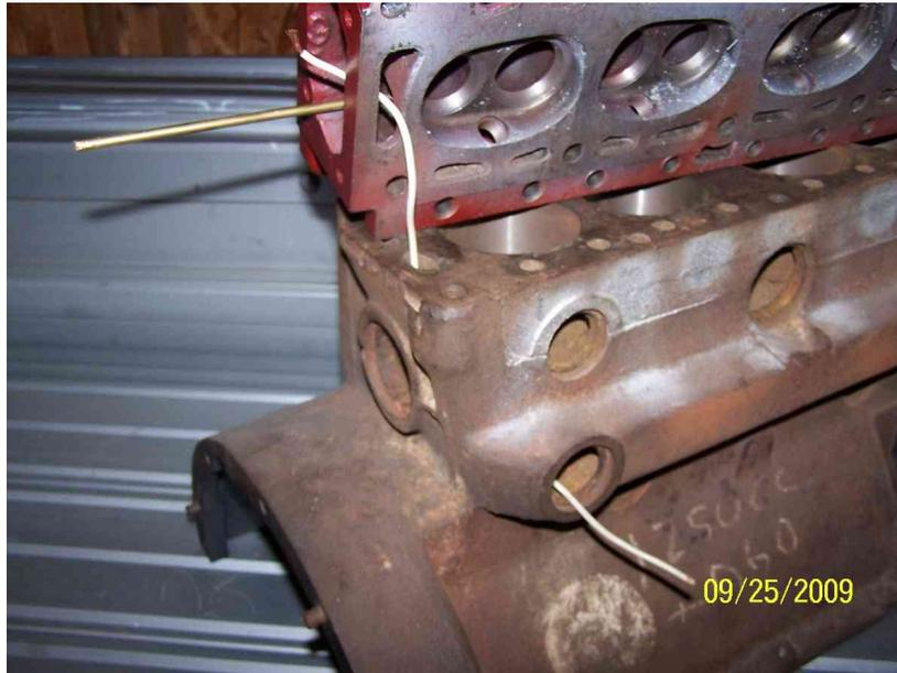
This passage is connected to the small openings (round or banana) that come up from the block...this is the thermo-siphon portion of the cooling system. The hot water/air rising from the internals of the block are mixed with the cooler water coming from the radiator and circulated around the head as it moves forward to the thermostat.
