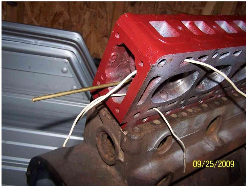
In this next photo I've inserted a brass rod all the way through the head to illustrate that there's an unbroken water passage from front to rear. Again, as the heat and hot water rises from the block it's picked up by the cooler water passing through the head on its way to the radiator.
