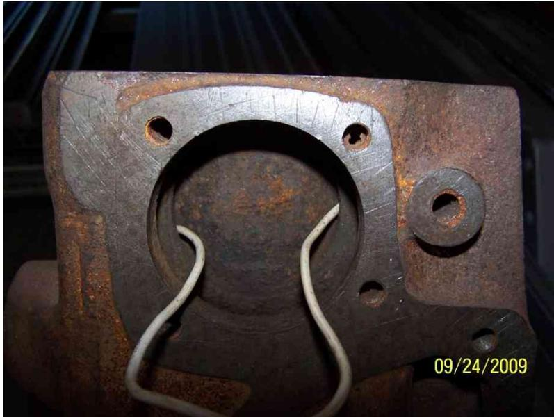
This next photo shows the larger passage at the bottom of the water pump area. This passage connects to the square protrusion on the side of the block that is normally hidden under the intake and exhaust manifolds. This passage carries the water from the water pump to the back of the block.
