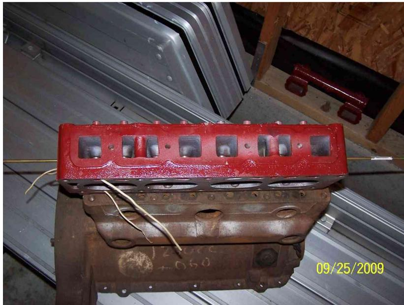
Now some photos to show how the rest of the cooling system is connected. With the exception of the square front to back passage the rest of the block is basically a water tank. As it heats the hotter water rises to the top of the block. This first photo shows how one of the small passages behind the water pump is connected to the front core plug and to the rest of the block.
