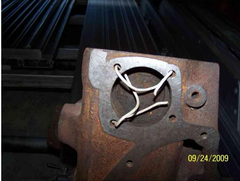
Inside the block around the water pump there are three passages. These first two that I've put the wire in are part of the thermo-siphon system. There would be little circulation action felt in this area because these passages are behind the impeller. I imagine these are there to help the block fill with water when the engine is cold and to let some hot water mix with the cooler water when the engine is running.
