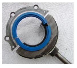
Be sure to lightly coat the seal lip with lubricant to avoid dry burn on start up.
