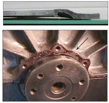
Note gap where oil could leak past when warped cover and not enough RTV was used.
