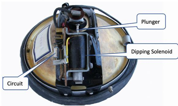
The Dipping Headlight was a device attached to the back of the nearside headlight reflector. It consisted of the bracket, four electrical connections, a solenoid with a plunger, a fuse, a resistor and two contact switches. When at rest (both contacts closed), a spring on the bracket keeps the plunger pulled out from the solenoid
