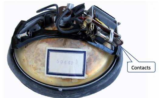
The dipping headlight was only installed on cars manufactured in 1936 (they were also used on the VA). In 1936, England passed a law outlawing the dipping unit from 1937 onward, so if you have one it's rather rare.
