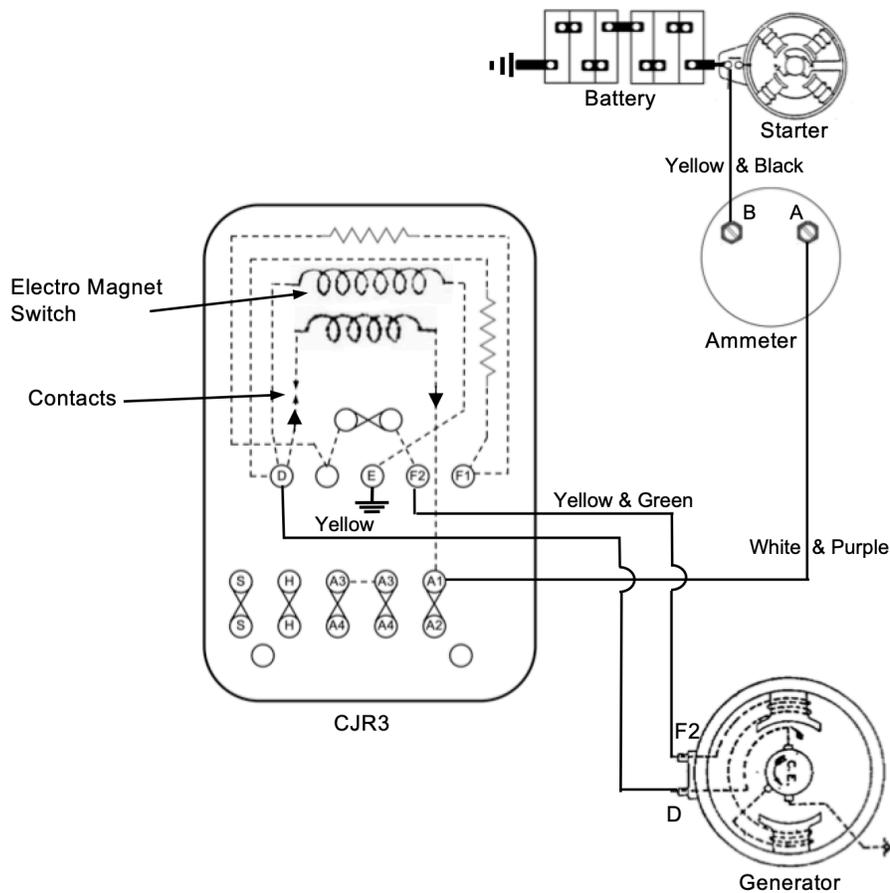
The other major function of the Cut-Out is protecting the Battery. When the Generator fails to produce enough power, either by slower speeds or failure, then the Contacts will open. If this did not happen, then power from the Battery would flow backwards through the system. From the Battery to the Starter Switch, across the Ammeter, to the CJR3 Terminal A1, then the D terminal and back to Generator and to the ground. This would result in draining the Battery.
