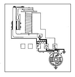
Power from the Generator falls off as soon as the circuit is broken. The reduced power then causes the electro-magnet to lose power. The magnetic pull is reduced and the Armature (3) is released from the magnet and the contacts are joined again reconnecting the D/F circuit. Then the whole cycle begins again. This entire process repeats between 60 and 100 times per second. The result of all this is a smooth regulated power flow from the Generator.
