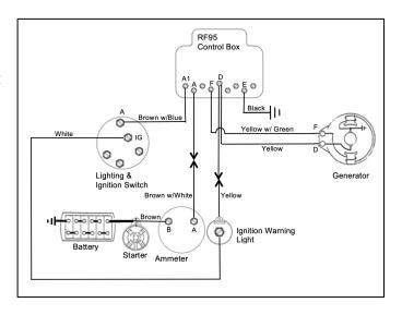
If the engine is not running or running slow, and therefor little or no power is being produced by the Generator, then electricity will flow through the circuit, from the battery to the RF95 Control Box and the light will come on being powered by the battery. When the car starts, and the generator produces enough output which is equal to or more than the battery output, then the two opposing flows will cancel each other out, no power will flow through the circuit and the light will go out.
