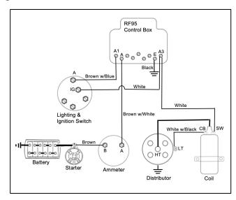
Power builds in the Magnetic Field, and when the Starter Switch is pulled the Distributor will rotate causing the Contact Points to open and close. This action will cause the Coil to perform in the manner noted above.
