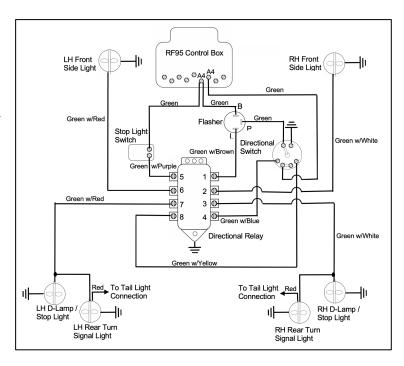
The P circuit continues to the Directional Switch where it powers the indicator light. The L circuit enters the Relay at connection 1 where it flows through the relay and out both 6 and 7 for a left-hand turn or 2 and 3 for a right-hand turn.
