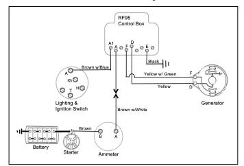
current flow, and the Ammeter will show neither negative nor positive charging. Output from the Generator will, however, flow from Terminal A1 and then to connection A on the Lighting & Ignition Switch and on to various components by way of the IG, H and T connections.
