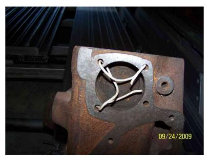
Inside the block around the water pump there are three passages. These first two that I've put the wire in are part of the thermo-siphon system. There would be little circulation action felt in this area because these passages are behind the impeller. I imagine these are there to help the block fill with water when the engine is cold and to let some hot water mix with the cooler water when the engine is running.
