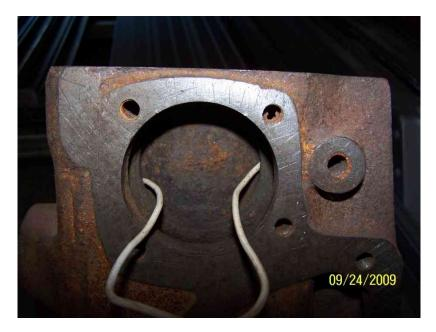
This next photo shows the larger passage at the bottom of the water pump area. This passage connects to the square protrusion on the side of the block that is normally hidden under the intake and exhaust manifolds. This passage carries the water from the water pump to the block of the block.
