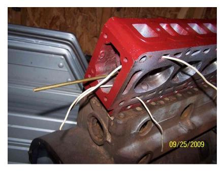
In this next photo I've inserted a brass rod all the way through the head to illustrate that there's an unbroken water passage from front to rear. Again, as the heat and hot water rises from the block it's picked up by the cooler water passing through the head on its way to the radiator.
