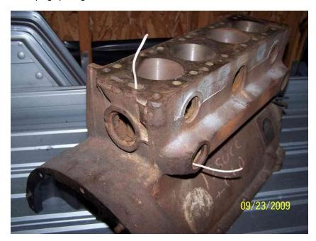
When the water exits the top of the block it goes into the head. As you can see the water comes in through the large opening at the rear of the head and into this chamber which connects to a passage that runs all the way through the head.
