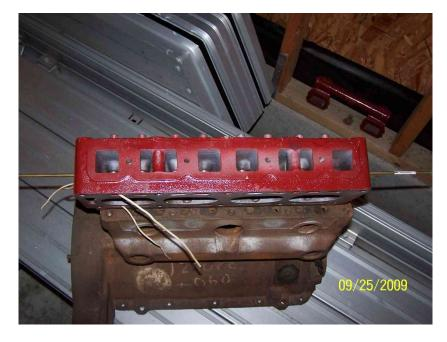
Now some photos to show how the rest of the cooling system is connected. With the exception of the square front to back passage the rest of the block is basically a water tank. As it heats the hotter water rises to the top of the block. This first photo shows how one of the small passages behind the water pump is connected to the front core plug and to the rest of the block.
