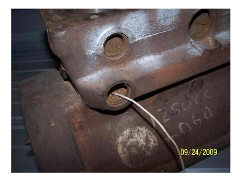
When the water reaches the rear of this passage it turns and goes up to the back of the head. There is no path into the block in this area except through the small hole behind the core plug. Remember that the water is relatively cool here so when it starts its journey through the head it will be extracting heat from this point forward. I could find no connection from this passage to the core plug opening on the back of the block.
