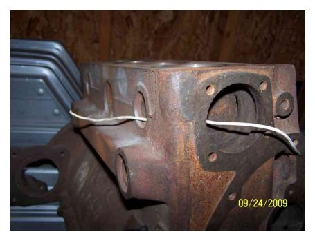
These next photos were taken to show that the block, with the exception of the piston cylinders is basically hollow and water is free to circulate (or stand) freely within it.
