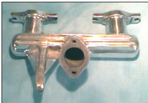
SPRITE MK1 OR A40 INLET MANIFOLD NO CNM 007
