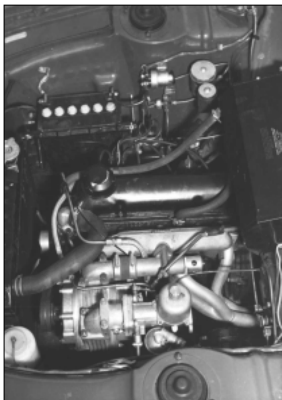
SHORROCK SUPERCHARGER C75B FITTED TO FORD 105E ENGINE
