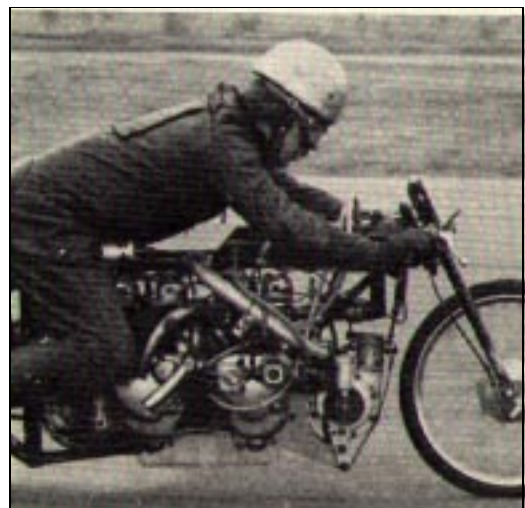
SHORROCK SUPERCHARGER C75B FITTED TO MOTOR BIKE
