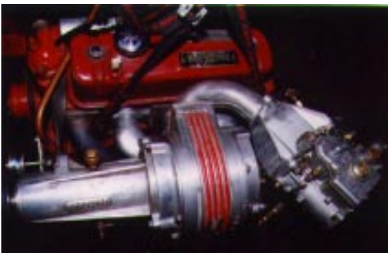
SHORROCK SUPERCHARGER C75B FITTED TO MGA 1500 ENGINE
