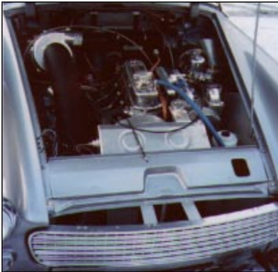
SHORROCK SUPERCHARGER C75B FITTED TO MK11 AUSTIN HEALEY SPRITE
