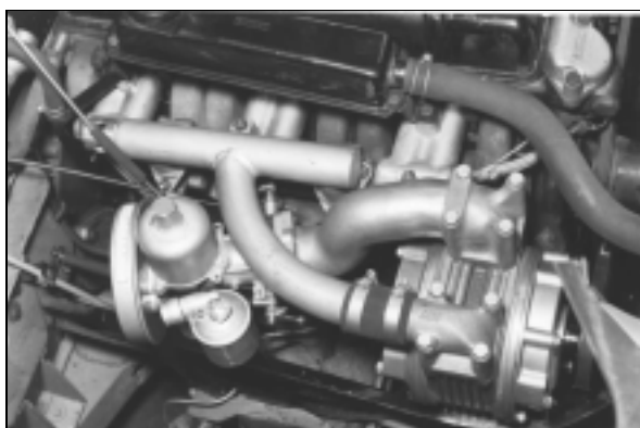
SHORROCK SUPERCHARGER C75B FITTED TO TRIUMPH VITESSE 6
