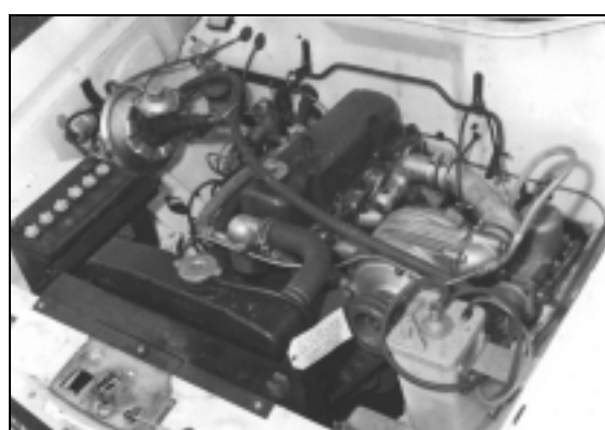
SHORROCK SUPERCHARGER C75B FITTED TO VAUSHALL VX 4/90
