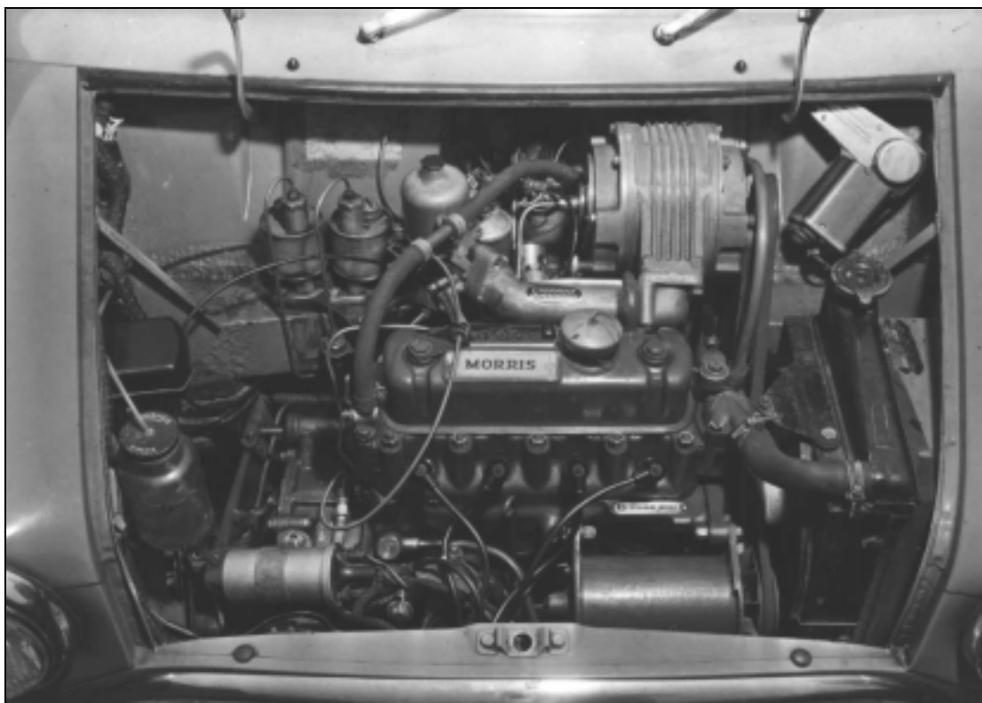
SHORROCK SUPERCHARGER C75B FITTED TO MINI ENGINE.
