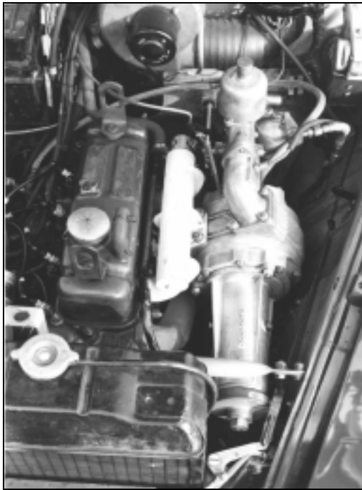
SHORROCK SUPERCHARGER LONG NOSE C75B FITTED TO RILEY 1.5 OR M.G. MAGNET
