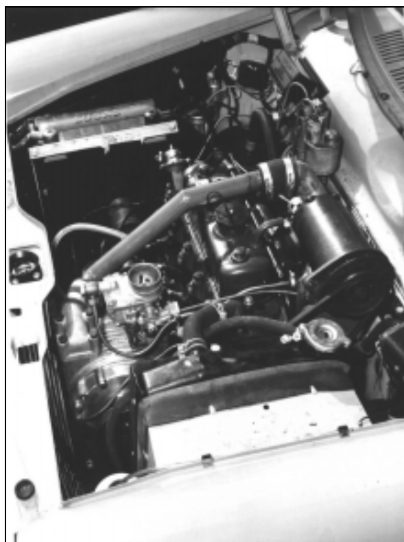
SHORROCK SUPERCHARGER C75B FITTED TO MORRIS 1100 ENGINE
